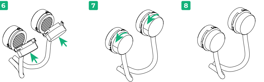
Reattach the silencer covers. Rotate counterclockwise to lock the latches in place. Complete
